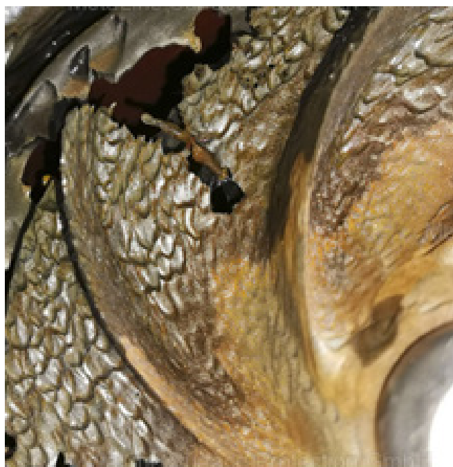
Fig-11: Effect-Impeller Without Coating, after 6 months in sewerage operation
