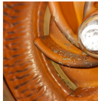
Fig-9 (B): Effect-Impeller Coated, after 6 months in sewerage operation
