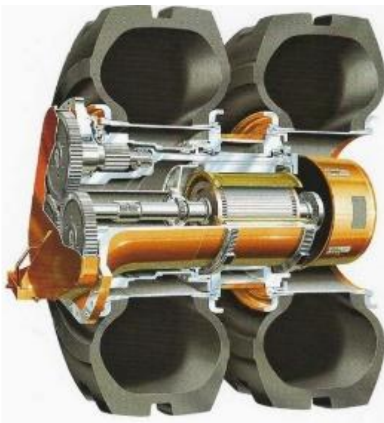
Fig-6: Electric drive of an off-highway, high-capacity dumper
